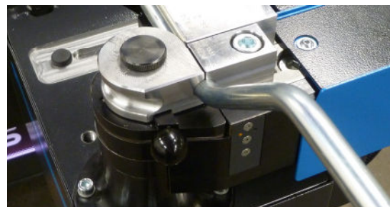
Fast and easy bending of steel pipe shapes up to Ø 16 mm.
